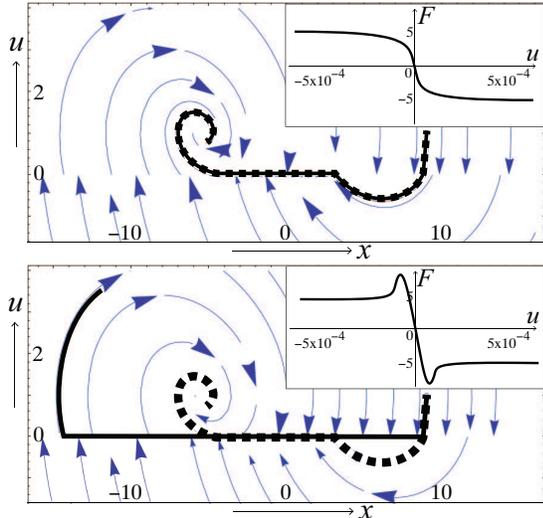
FIG. 2. Simulation with error (dotted path) and without error (full curve), using friction models  $F(u) = -\tanh(u/\varepsilon)$  (top) and  $F(u) = -(1 + 2\pi e^{-u^2/\varepsilon^2}) \tanh(u/\varepsilon)$  (bottom) shown inset.
